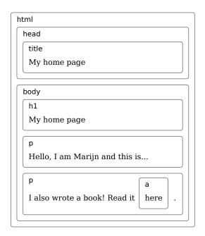
The data structure the browser uses to represent the document follows this shape. For each box, there is an object, which we can interact with to find out things such as what HTML tag it represents and which boxes and text it contains. This representation is called the *Document Object Model*, or DOM for short.
